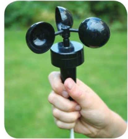
Figure 21.36 Measuring wind speed
